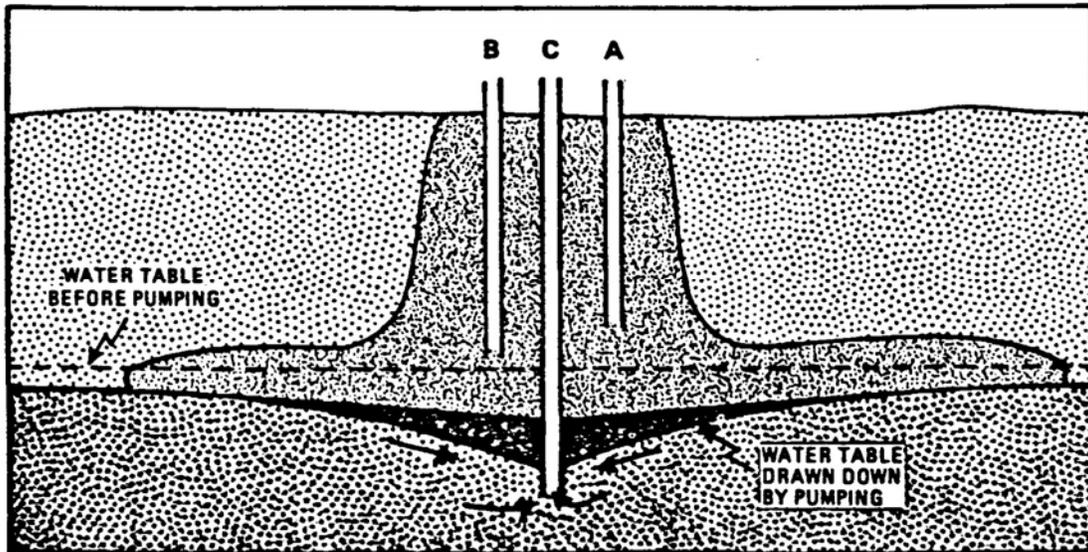
**Figure 10-11: Effect on Water Table of Pumping from Well C**
