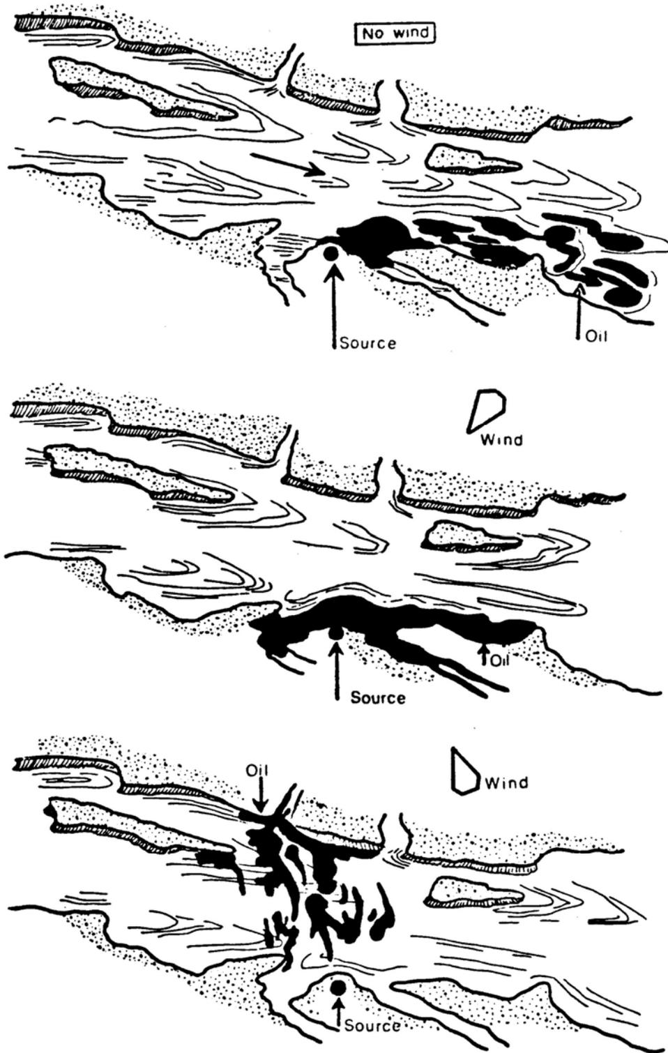
**Figure 7-5: Wind Effect on Oil Movement**
