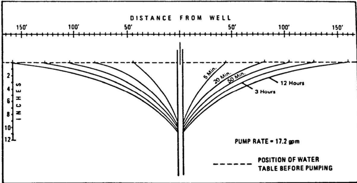
Figure 10-12: Diagrammatic Illustration of Development of a Cone of Depression Based on an Actual Aquifer Test
