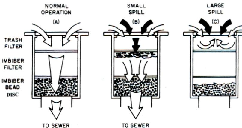
**Figure 6-7: Imbiber Beads<sup>®</sup> Gravity-Flow Drain Protection System—Operational Process**
