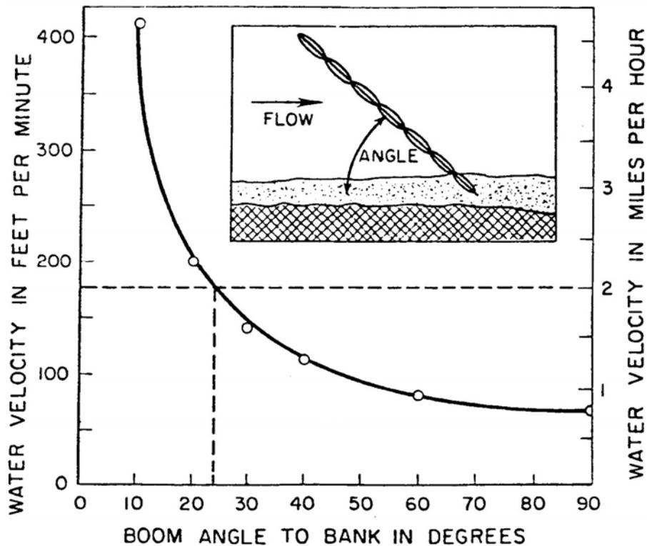
**Figure 7-9: Suggested Boom-to-Shoreline Angles for Different Current Velocities**
