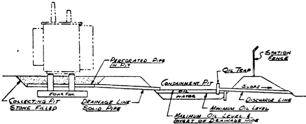
Figure 6-3: Cross Section of Oil Drainage System
