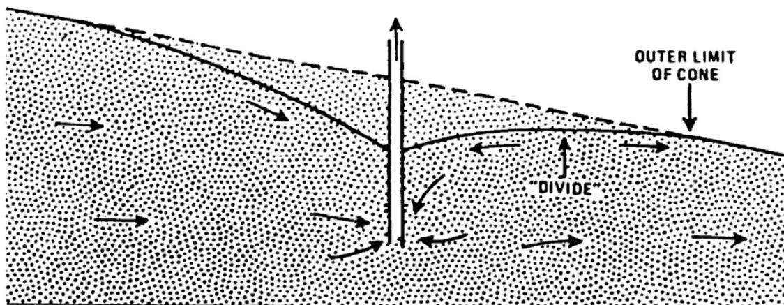
**Figure 10-14: Drawdown Configuration of Well Pumping From Inclined Water Table**
