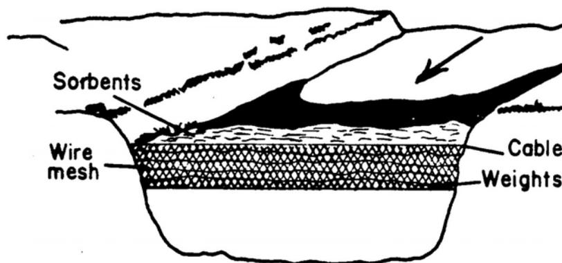
**Figure 7-15 : Cross Section of a Sorbent Fence**
