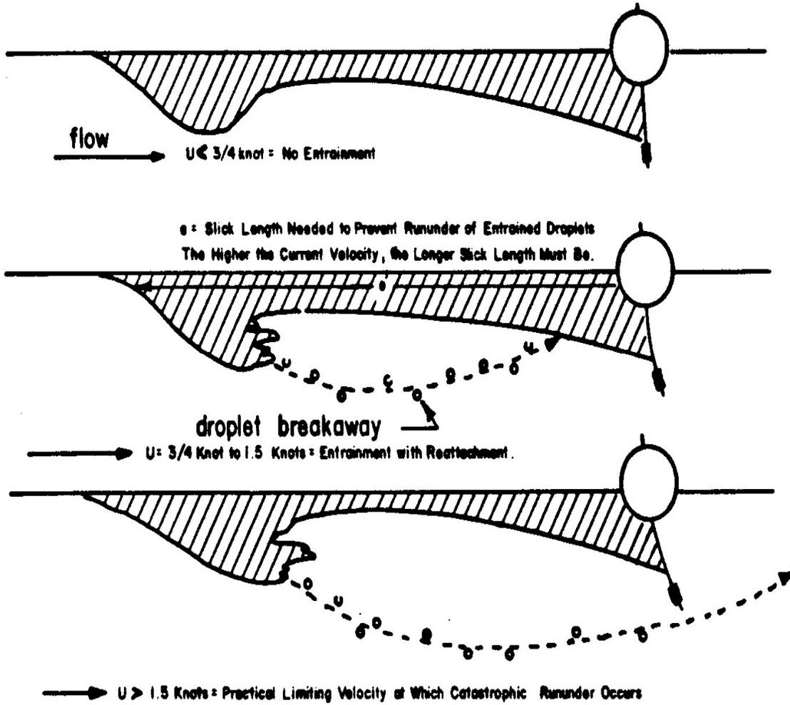
Figure 5-6: Entrainment Failure
