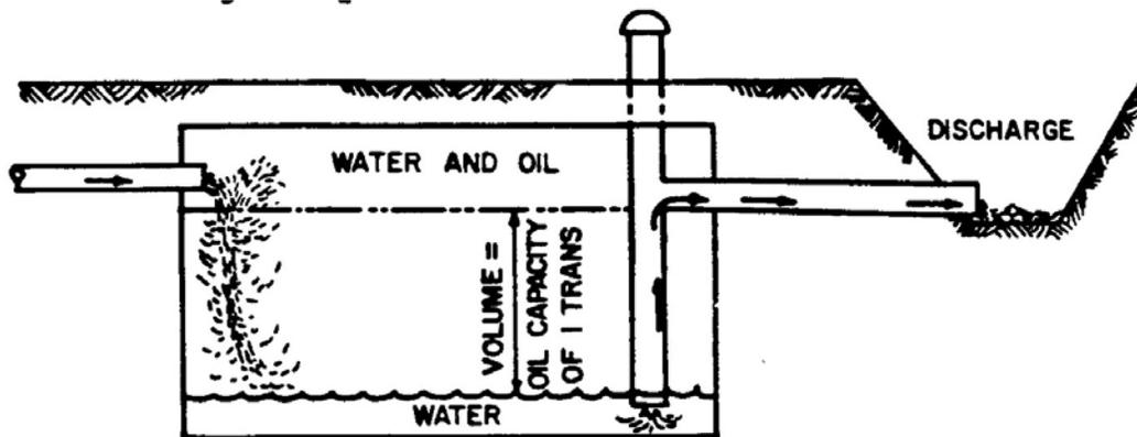
Figure 6-10: Typical Construction of Oil Separator Tank
